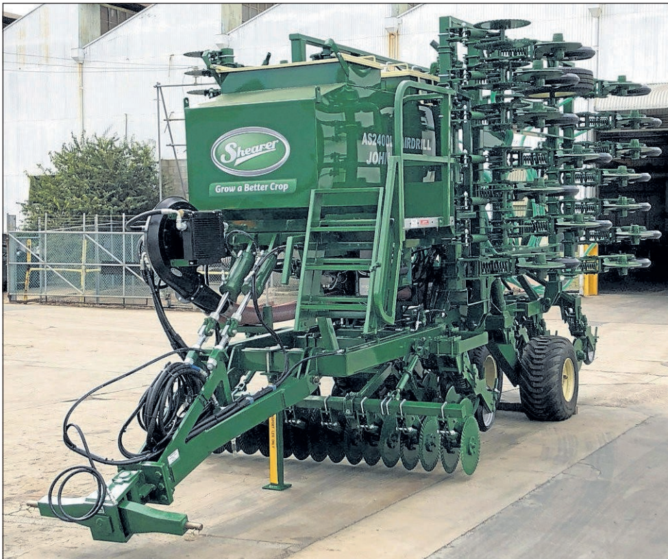
The distribution module of the John Shearer air drill is uniquely engineered to ensure it is simple to operate, easy to calibrate sowing rates and effortless to clean out.
